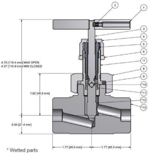
Lubrication: Molybdenum disulfide with soft metallic fillers
