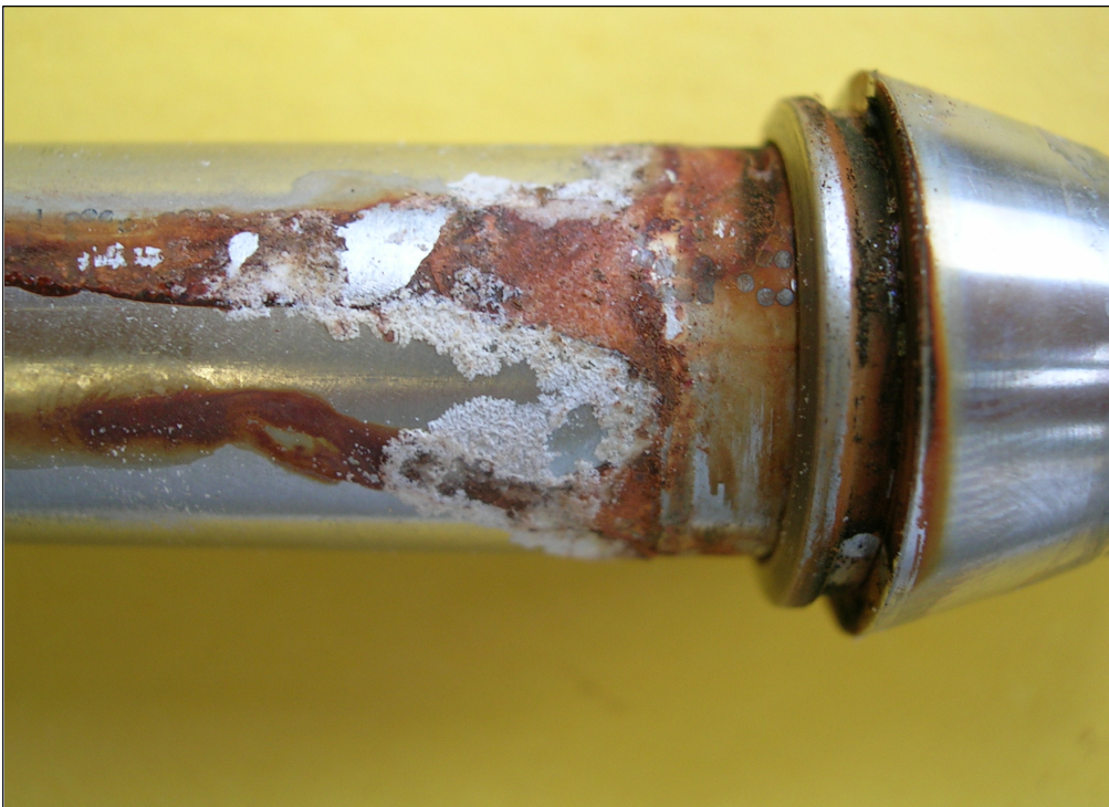
Figures 5 and 6 – Tube Fitting Assemblies with Stainless Steel 316 Tubing after 175h Exposure to Salt-Spray Test as per ASTM B117 Specification.
